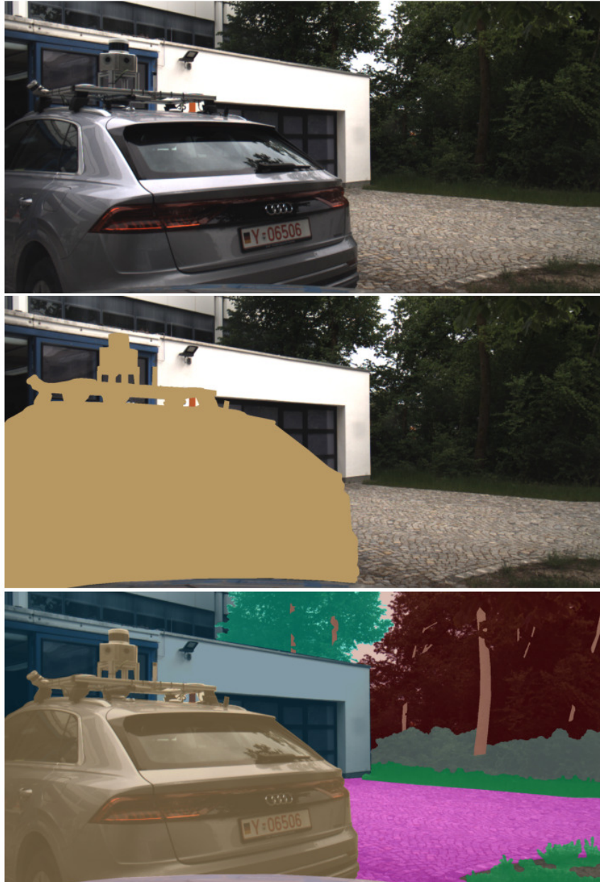
Figure 12.2: A roof construction as well as cameras, LiDAR sensors and antennas are also labeled as part of the car (■).
