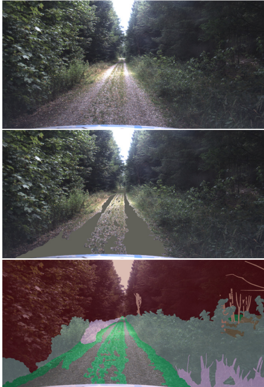
Figure 24.2: Annotation examples of gravel (■). Notice that the grass patches in the middle of the gravel road are annotated separately as low_grass (■).
