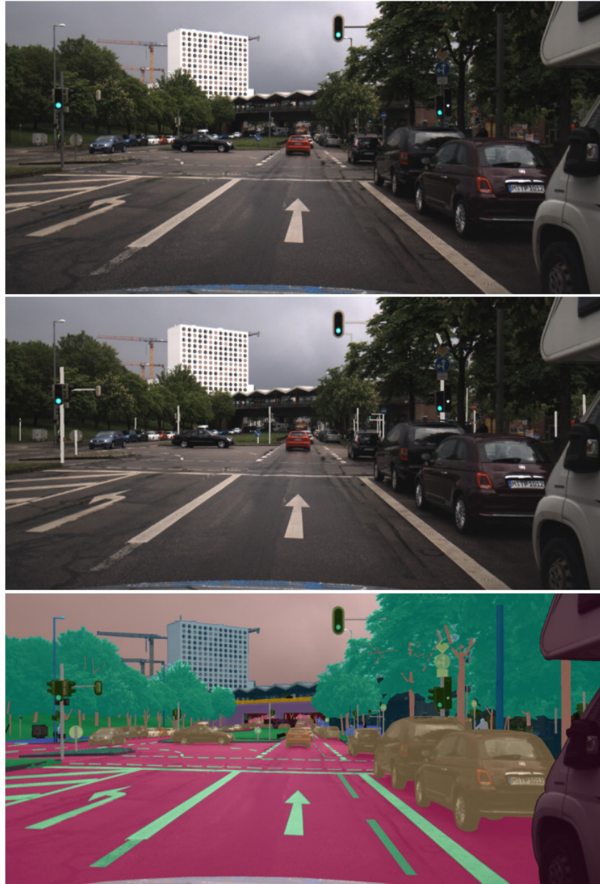
Figure 44.2: Example of annotated poles by the traffic lights (■) and the difference to street lights (■).
